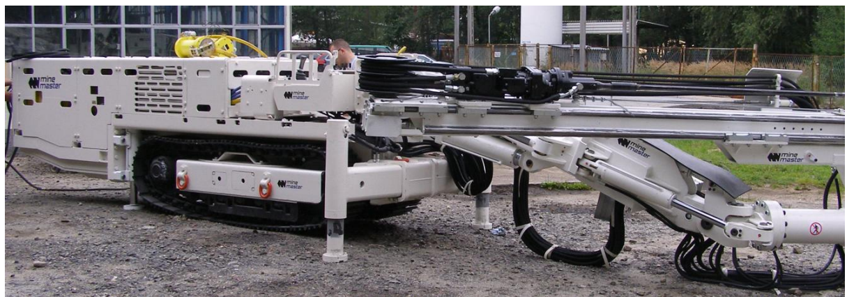
Face drill rig Face Master 1.8W - Caterpillar carrier
