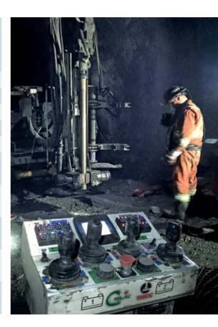
A self-propelled Production Master 2.3 long hole drill rig is designed for drilling parallel upholes and downholes as well as fans and rings in vertical or inclined planes. A top-hammer system gives the possibility of drilling in a range of 64-165 mm holes depending on the configuration. Easy to use positioning
